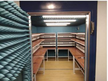
Anechoic chambers can range in size from a table top enclosure to a typical room, where engineers can walk in and work, to a space as large as an aircraft hanger.
